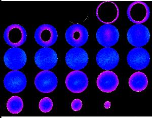
This result shows a PLG-650 laser pulse being stepped through a 4 ns gate window generated by a PHOTEK GM200-3N gate unit on a PHOTEK MCP118 image intensifier. Each step represents an extra 200 ps delay on the laser pulse.
