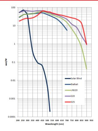
The above curves represent the broad spectral response that you would expect to achieve with Photek's range of Gen II photocathodes. Please note that input window material and fast gating requirement will affect overall sensitivity.
