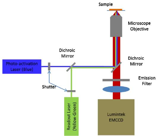
be focussed onto the sample, stimulated the activated dyes to fluorescence. The red fluorescence light is passed through a dichroic mirror, filtered to remove extraneous light and imaged onto a Lumintek MP Vision EMCCD camera. After photo-bleaching has deactivated some of the fluorescent dyes, the activation laser is used to activate additional dyes. This process is continued until sufficient signal has been obtained to reconstruct a super resolution image.
