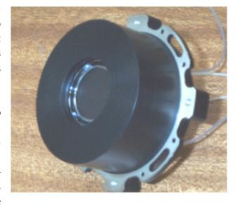
and operate over a wide range of temperatures and are subjected to both thermal and vacuum cycling. The use of low outgassing materials for encapsulation of the image tubes, which operate at high voltages, is critical both to the tubes operation and to prevent potential contamination of the sensitive FUV optics. Above is an image of the ruggedized GUVI photon counting imager.
